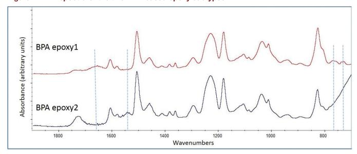
The major peak patterns are the same. Regions in which the two spectra differ are indicated by dashed lines. The upward slope at the right-hand side of the BPA epoxy2 spectrum is from an inorganic oxide such as titanium dioxide or zinc oxide.
